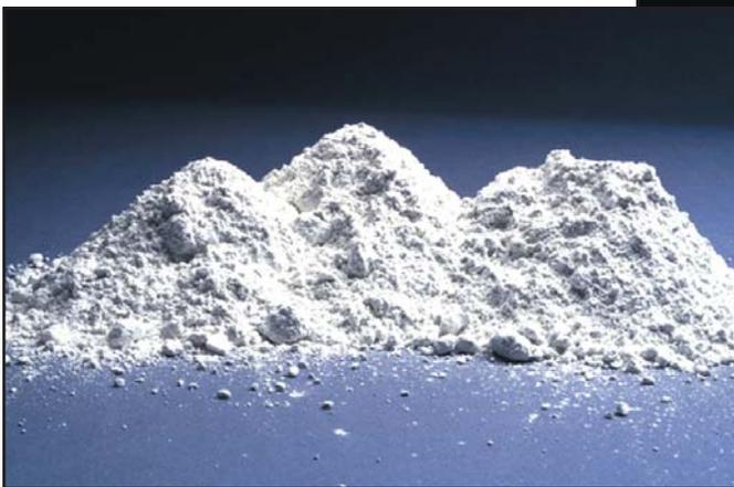
**Figure 10.** White portland cement is the key ingredient to making white and colored concrete. For maximum brightness, white or other light-colored fine and coarse aggregates should be used. (69636)
