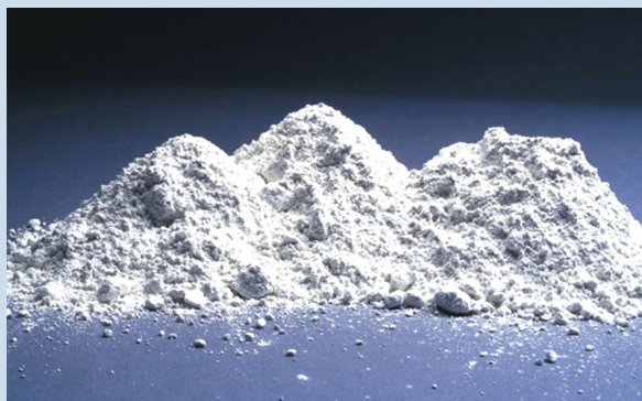
Figure 2. White cement provides a neutral base for mortars whether they are white or tinted. The sand can have a tinting effect on mortar, so it should also be carefully selected for color.
